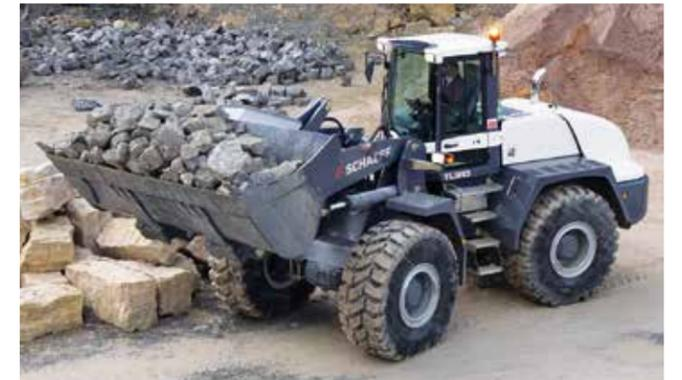
High tear-out and lifting forces thanks to a combination of high stability and parallel and Z-kinematics.
